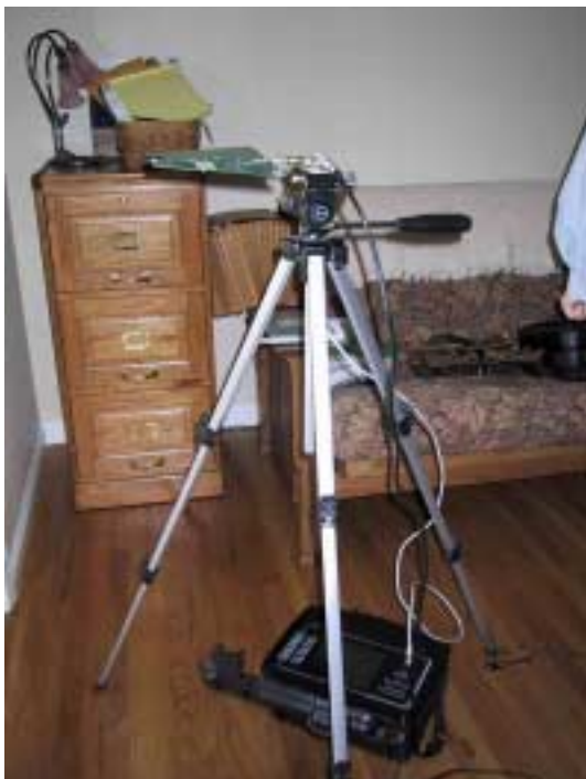
Figure 2: Typical indoor set-up, using an experimental antenna and Sencore AT-986
